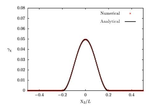
Fig. 4: Analytical (black line) and finite element (red crosses) solutions of differential equation (38) with a linear negative hardening ( $H = -250 \,\mathrm{MPa}$ ) at  $\overline{F}_{12} = 1\%$
