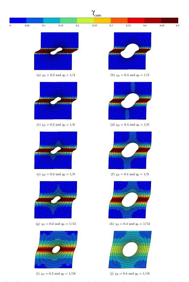
Fig. 9: Finite element results showing the interaction of a slip band and a void in a unit cell under average shear at  $\overline{F}_{12} = 0.15$
