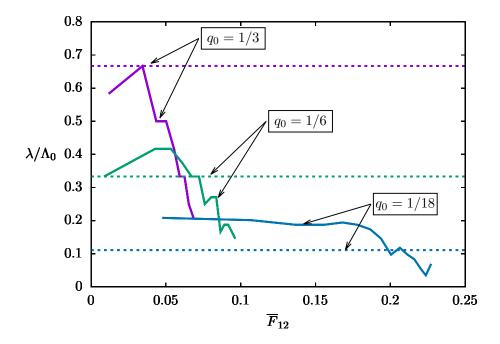
Fig. 11: Normalized localization slip band width  $\lambda$  as a function of  $\overline{F}_{12}$  for three different values of parameter  $q_0$  and for  $\chi_0 = 0.4$ . Dashed lines represent the normalized width equal to four times the initial mesh size.
