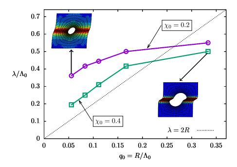
Fig. 12: Normalized localization slip band width  $\lambda$  as a function of  $q_0$  for two different void volume fractions at the overall shear value  $\overline{F}_{12} = 0.025$ . Insets correspond to snapshots of figure 9i (left) and 9b (right) at  $\overline{F}_{12} = 0.15$
