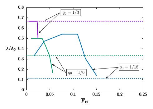
Fig. 10: Normalized localization slip band width  $\lambda$  as a function of  $\overline{F}_{12}$  for three different values of parameter  $q_0$  and for  $\chi_0 = 0.2$ . Dashed lines represent the normalized width equal to four times the initial mesh size.
