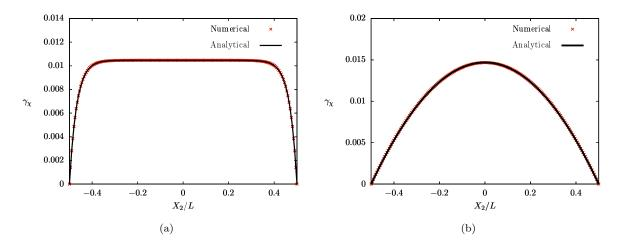
Fig. 3: Analytical (black line) and finite element (red crosses) solutions of differential equation (38) with: (a) a strictly positive linear hardening ( $H = 1000 \,\text{MPa}$ ) and (b) perfect plasticity ( $H = 0 \,\text{MPa}$ ) at  $\overline{F}_{12} = 1\%$
