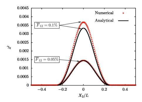
Fig. 6: Analytical (black line) and finite element (red crosses) solutions of differential equation governing  $\gamma_{\chi}$  at  $\overline{F}_{12} = 0.05\%$  and  $\overline{F}_{12} = 0.1\%$ , when considering the non-linear softening behaviour (63) and the constitutive function (69) for  $A(\gamma_{cum})$
