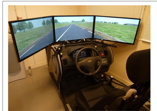
FIGURE 1 | Driving simulator setup: the driving scene is displayed on three screens. The Eye Tracker was composed of four cameras.
