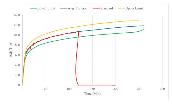
Figure 2: Actual Furnace Average Temperature / Time curve.
