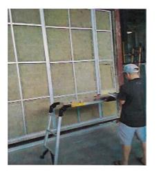
Plate 1. Before the test. (during the construction showing the rockwool infilled and studs)
