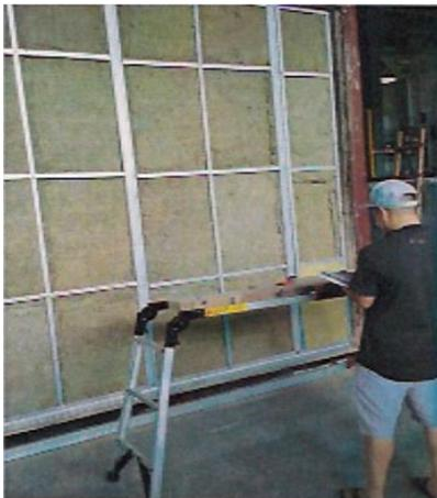
Plate 1. Before the test. (during the construction showing the rockwool infilled and studs)
