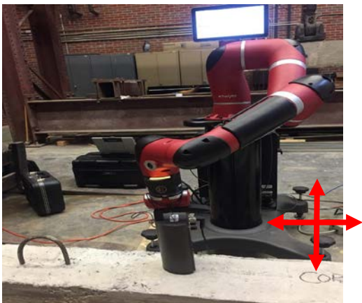
Figure 4. Robotic Impact Echo (IE)
