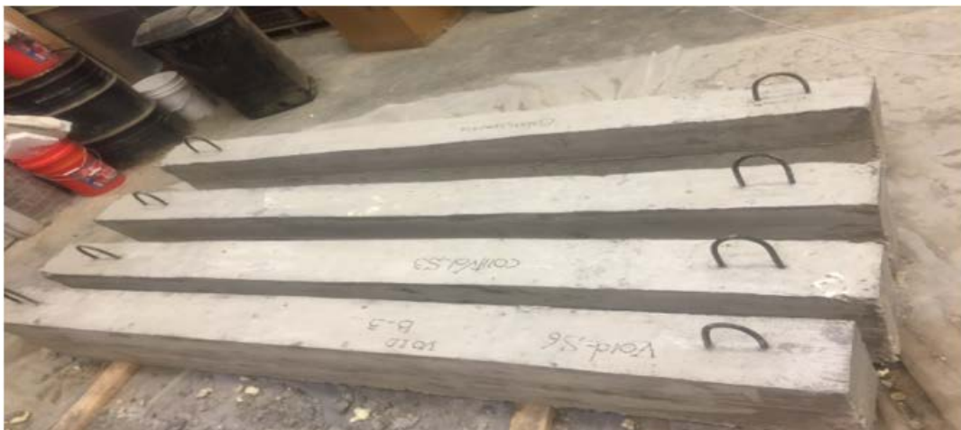
Figure 1. RC Beams uses for the NDE Research
