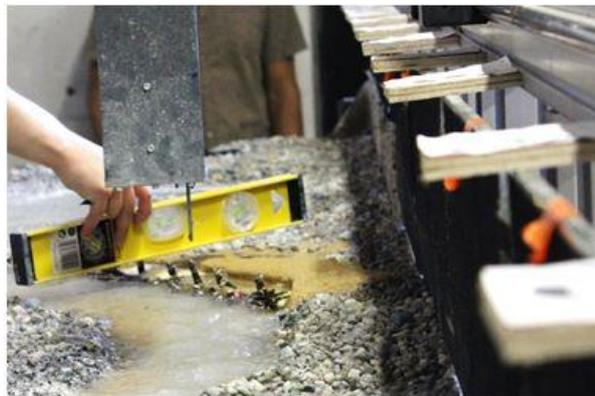
Figure 4: Channel width and channel depth measurement (point gauge), ground control point targets can be seen on the right-hand side of the picture.
