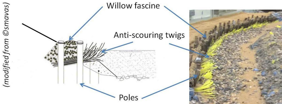
Figure 3: Toe protection with twigs: profile sketch for construction and small-scale model
