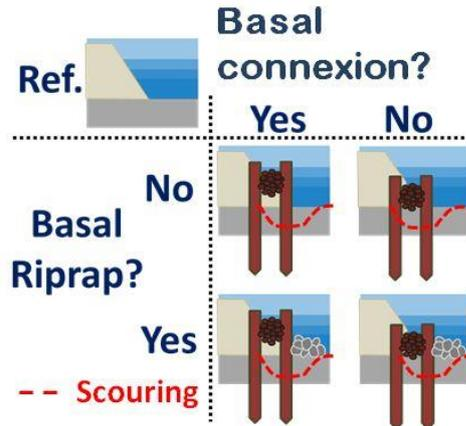
Figure 2: Tested configuration of different connection and protection scenarios between the erodible bed and the flow. Grey material represents the bed, a relatively coarse mixture, fixed (set 1) or mobile (set 2). The beige material behind the fascine represents highly erodible fine sand. The red dashed line represents scouring in the second set of experiments
