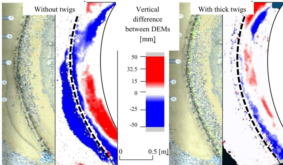
Figure 13: Diachronic analysis of bed topography changes for two runs with and without twigs. Erosion (in blue) is substantially reduced in presence of twigs.
