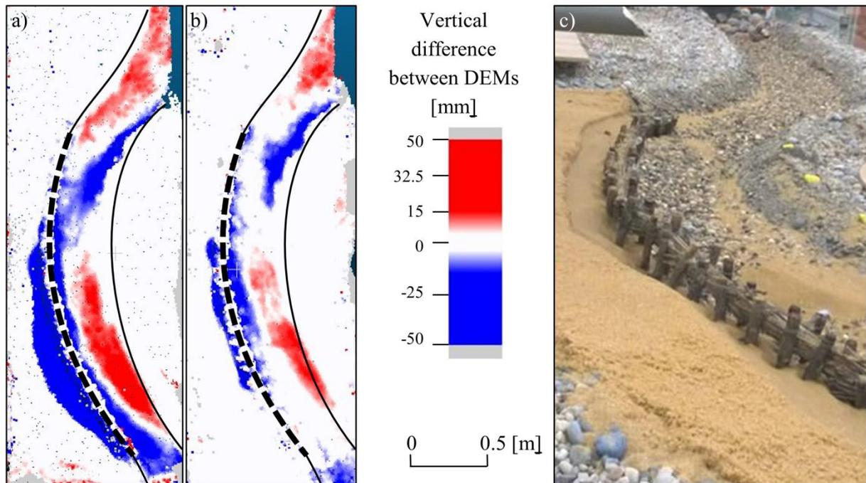
Figure 10: Diachronic analysis of bed topography evolution for two repeated runs with a mobile bed (a and b). Erosion (in blue) reached several centimetres below the fascine while deposition (in red) can be observed outside the bend as shown in (c), a photo of the final state of another run.
