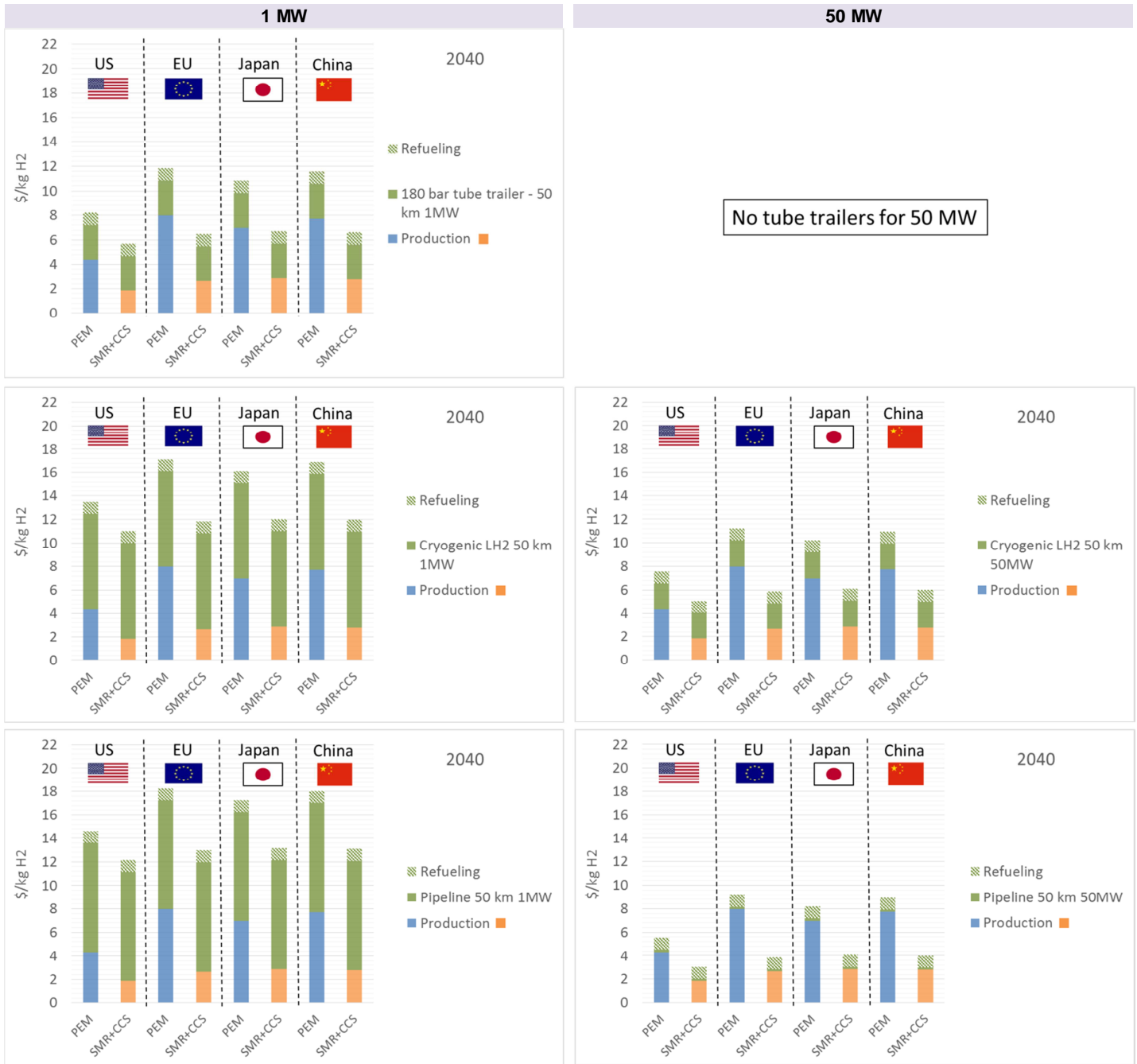
Figure 9: Hydrogen cost at the pump for the centralized case study in 2040 (left column 1 MW, right column 50 MW of throughput capacity, each line corresponds to a delivery pathway)
