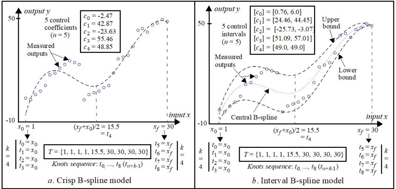
Fig. 35: B-spline model illustration (5 control coefficients)
