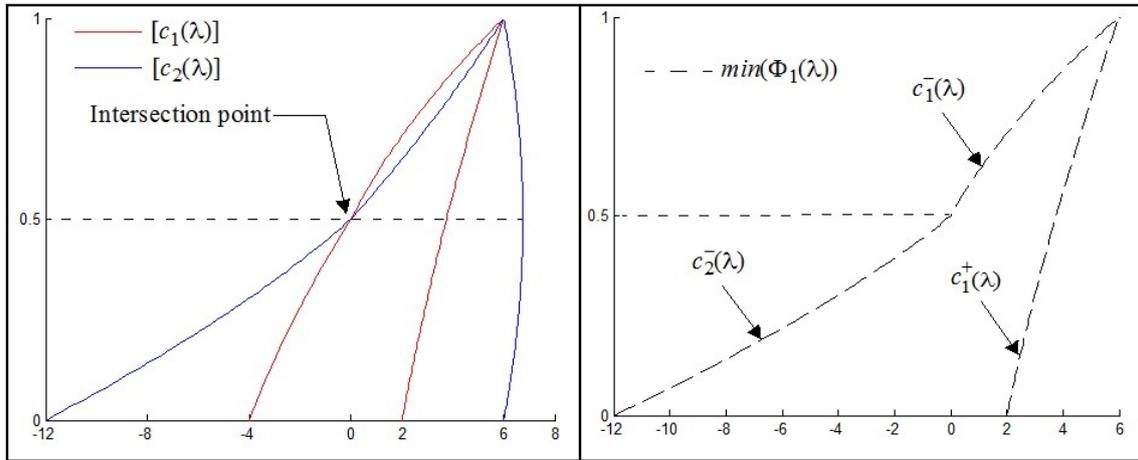
Fig. 14: Computational principle of  $\min(\Phi_1(\lambda))$
