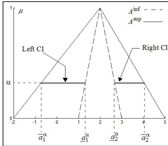
Fig. 17:  $\alpha$ -plane principle on T2FI  $\tilde{A}$
