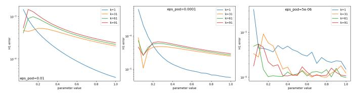
Figure 12: Test case (c) : Relative  $H^1$ -error  $e^k(\mu)$  for some time nodes  $k \in \mathbb{K}^{\text{tr}}$ and M = 121. Left:  $\epsilon_{\text{POD}} = 10^{-2}$  (N = 3). Middle:  $\epsilon_{\text{POD}} = 10^{-4}$  (N = 7). Right:  $\epsilon_{\text{POD}} = 5.10^{-6}$  (N = 11).
