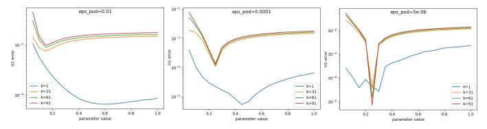
Figure 13: Test case (d) : Relative  $H^1$ -error  $e^k(\mu)$  for some time nodes  $k \in \mathbb{K}^{\text{tr}}$ and M = 121. Left:  $\epsilon_{\text{POD}} = 10^{-2}$  (N = 3). Middle:  $\epsilon_{\text{POD}} = 10^{-4}$  (N = 7). Right:  $\epsilon_{\text{POD}} = 10^{-6}$  (N = 11).
