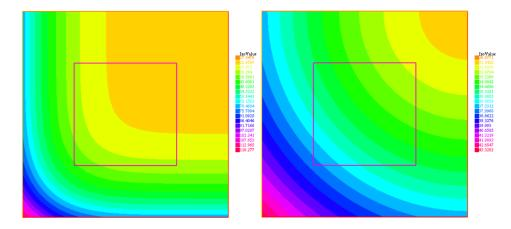
Figure 5: Test cases (a) and (b) : HF solutions for the bk model with Neumann boundary conditions. Left:  $\mu = 1$  in  $D_{\text{uni}}$  (values from 17.3°C to 118.3°C). Right:  $\mu = 20$  in  $D_{\text{uni}}$  (values from 30.7°C to 43.3°C).
