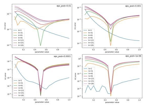
Figure 9: Test case (b) : Relative  $H^1$ -error  $e^k(\mu)$  for some time nodes  $k \in \mathbb{K}^{\text{tr}}$ and M = 676. Top left:  $\epsilon_{\text{POD}} = 10^{-2}$  (N = 5). Top right:  $\epsilon_{\text{POD}} = 10^{-3}$  (N = 7). Bottom left:  $\epsilon_{\text{POD}} = 10^{-4}$  (N = 10). Bottom right:  $\epsilon_{\text{POD}} = 10^{-6}$  (N = 15).
