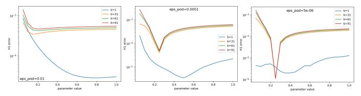
Figure 14: Test case (d) : Relative  $H^1$ -error  $e^k(\mu)$  for some time nodes  $k \in \mathbb{K}^{\text{tr}}$ and M = 676. Left:  $\epsilon_{\text{POD}} = 10^{-2}$  (N = 3). Middle:  $\epsilon_{\text{POD}} = 10^{-4}$  (N = 7). Right:  $\epsilon_{\text{POD}} = 5.10^{-6}$  (N = 11).
