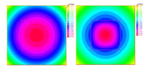
Figure 11: Test cases (c) and (d) : Left: HF solution for the bk model (values from 17.80°C to 18.25°C). Right: Synthetic true solution using a bi-material plate (values from 17.90°C to 18.23°C).
