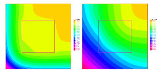
Figure 7: Test case (b) : Synthetic true solutions with Neumann boundary conditions. Left:  $\mu = 1$  in  $D_{\text{syn}}(\mu)$  (values from 17.4°C to 117.9°C). Right:  $\mu = 20$  in  $D_{\text{syn}}(\mu)$  (values from 29.8°C to 44.3°C).
