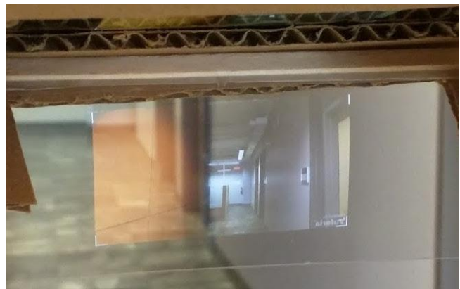
Figure 8. View of the camera’s phone projected to the plastic sheet of CARTON
