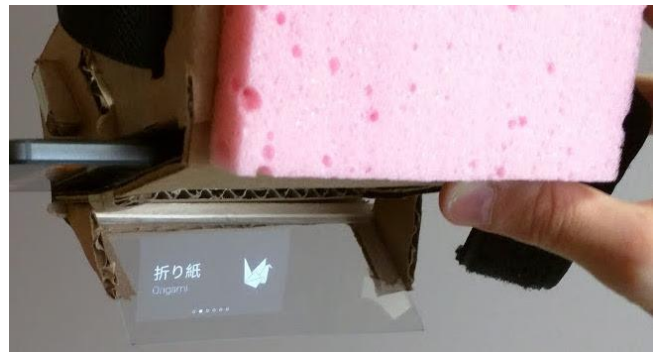
Figure 2. Overview of a mobile application projected to the plastic screen
