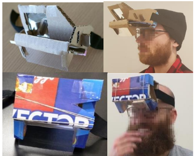
Fig. 1. Top: first version of the headset. Bottom: second version of the headset, easier to build with safer tools and material.
