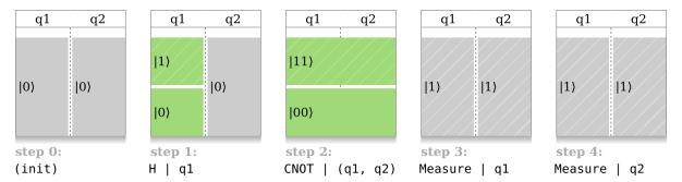
Figure 5: Visualization of the creation and the measurement of a Bell pair, using the proposed approach.
