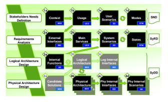
Figure 01: SysCARS System Engineering Process
