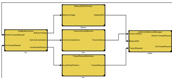
Figure 10: Simulink Controller Architecture (Dataflow)
