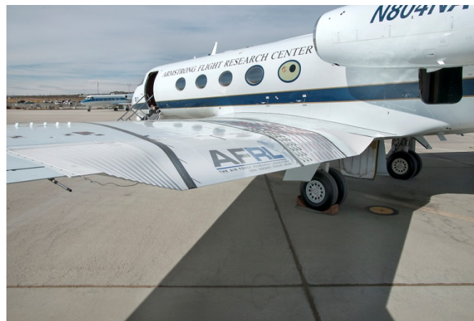
Figure 7: ACTE flaps on NASA's Gulfstream III aeronautical test bed [12].
