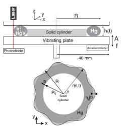
FIG. 1: Top: Experimental setup. Plate forcing:  $A \sin (2\pi ft)$ . Bottom: top view of fluid torus deformations (mode 7).
