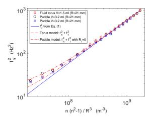
FIG. 4: Resonance frequency  $f_n$  of mode n vs  $n(n^2 - 1)/R^3$  for a fluid torus ( $\Diamond$ ) or for two distinct sets of puddle for the same control parameters ( $\circ$ ,  $\Box$ ). R = 21 mm. n = 5 to 25. Solid line corresponds to Eq. (1), dashed and dash-dotted lines to  $f_n^2 + f_1^2$  [from Eqs. (1) and (2)] for a torus and a puddle  $(R_i = 0)$ , with  $f_1 \simeq 3.6$  and 2.1 Hz, respectively.
