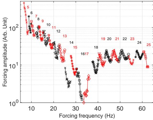
FIG. 3: Phase diagram of the lobes occurring on a vibrating torus showing the resonance tongues from  $n = 5$  to 25. To better distinguish successive tongues, the corresponding data and mode number  $n$  are colored alternatively in black and red (light-grey).  $V = 1.5$  mL.
