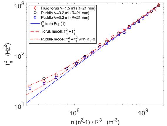
FIG. 4: Resonance frequency  $f_n$  of mode  $n$  vs  $n(n^2 - 1)/R^3$  for a fluid torus ( $\diamond$ ) or for two distinct sets of puddle for the same control parameters ( $\circ$ ,  $\square$ ).  $R = 21$  mm.  $n = 5$  to 25. Solid line corresponds to Eq. (1), dashed and dash-dotted lines to  $f_n^2 + f_1^2$  [from Eqs. (1) and (2)] for a torus and a puddle ( $R_i = 0$ ), with  $f_1 \simeq 3.6$  and 2.1 Hz, respectively.
