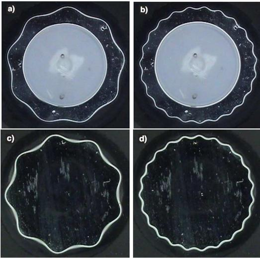
FIG. 2: Top view of the azimuthal pattern displayed at the periphery of a torus (a, b) and of a puddle (c, d) of mercury for  $f = 16.4$  Hz (a, c) and  $f = 43$  Hz (b, d). The corresponding numbers  $n$  of lobes, oscillating radially at  $f/2$  are  $n = 9$  (a, c) and  $23$  (b, d), respectively. Grey areas correspond to the solid cylinder (a, b). Torus or puddle diameter at rest  $\approx 42$  mm.  $V = 1.5$  mL (a, b).  $V = 3.2$  mL (c, d).
