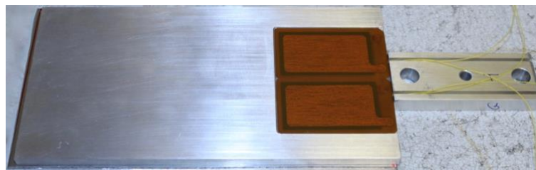
Figure 4: Flat plated equipped with the piezoelectric patches
