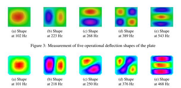
Figure 4: Measurement of five operational electrical current shapes in the network
