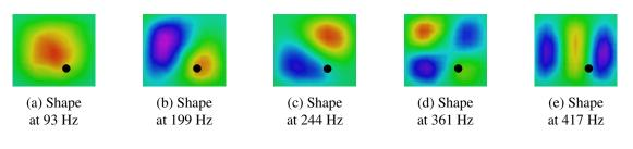
Figure 12: Measurement of five operational deflection shapes of the plate when a 207 g mass (in black) is added
