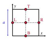
Figure 1: Discretization grid, where I, B, L, R, T refer to the central, bottom, left, right and top positions, respectively
