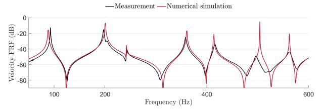
Figure 11: Experimental and simulated FRFs with short-circuited piezoelectric patches and an added mass
