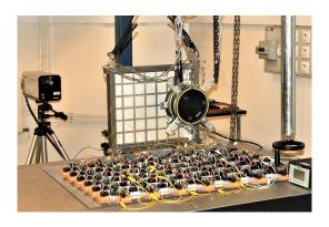
Figure 7: Setup including the plate covered with piezoelectric transducers, a shaker, a laser vibrometer and the plate electrical analogue
