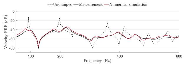
Figure 14: Experimental and simulated FRFs when the non-periodic plate is coupled to its electrical analogue
