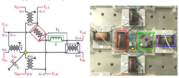
Figure 2: Scheme and picture of the electrical analogue of a square plate, which highlight the central transformer in red, a side transformer in blue, the inductance in green, and the capacitance connection in yellow
