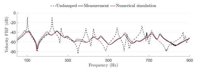
Figure 10: Experimental and simulated FRFs when the plate is coupled to its electrical analogue
