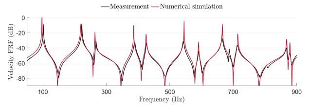
Figure 9: Experimental and simulated FRFs with short-circuited piezoelectric patches
