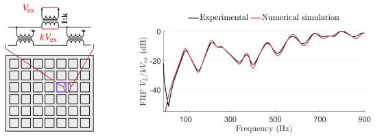
Figure 5: Schematic representation of the excitation setup for the measurement of network modes
