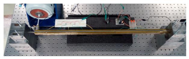
Figure 1: Beam covered with an array of piezoelectric patches; half of the patches are connected to a single resonant shunt for vibration damping of the first mode [5].
