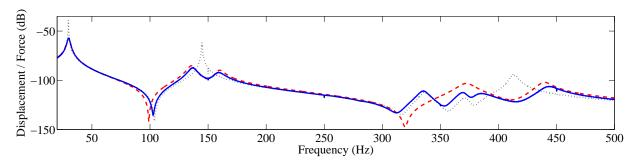
Figure 14: Frequency response functions at low excitation levels with short-circuited patches  $(\cdots)$  and with coupling to the analogous electrical network: model (--), experiment (--).
