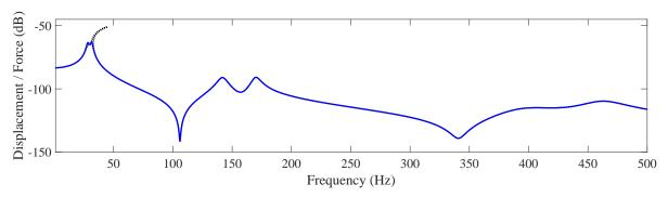
Figure 7: Simulated frequency response function of the nonlinear beam for F = 0.8 N without nonlinear capacitance (...) and with nonlinear capacitance (...)
