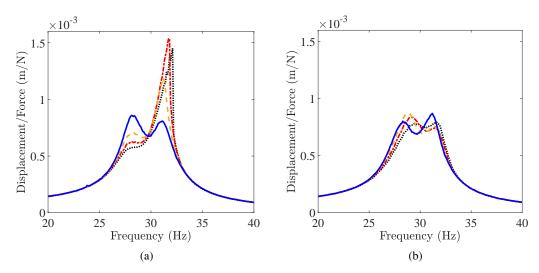
Figure 3: Experimental frequency response functions for various forcing amplitudes, F = 0.2 N (-), F = 0.4 N (-), F = 0.6 N (-) and  $F = 0.8 \text{ N } (\cdots)$  (a) linear shunt, (b) nonlinear piezoelectric tuned vibration absorber [5].
