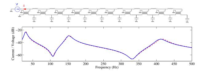
Figure 10: Experimental (—) and simulated (—) frequency response functions of the electrical network.
