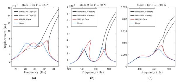
Figure 8: Simulated frequency responses for the first three modes – (a) mode 1 for F = 0.8 N, (b) mode 2 for F = 80 N, (c) mode 3 for F = 1800 N.
