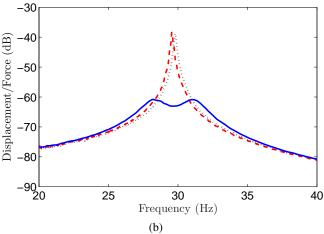
Figure 2: Piezoelectric tuned vibration absorber – (a) physical inductor, (a) experimental frequency response function around the first mechanical resonance, with short circuit  $(\cdots)$ , with open circuit  $(\cdots)$  or with an optimal linear shunt (-).
