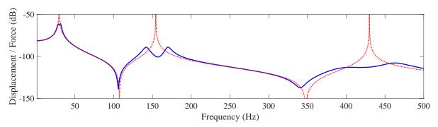
Figure 6: Simulated frequency response function of the beam with short-circuited patches  $(\cdots)$  and with the analogous electrical network (--).
