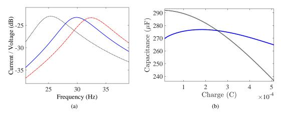
Figure 12: Choice of the capacitor at the end of the electrical network – (a) experimental frequency response function of the electrical network for various end-capacitors:  $166 \,\mu\text{F}(-\cdot-)$ ,  $266 \,\mu\text{F}(-\cdot)$  and infinite capacitance  $(\cdot\cdot\cdot)$ , (b) objective for the nonlinear capacitor  $(\cdot\cdot\cdot)$  and measurement on a physical capacitor  $(-\cdot)$ .
