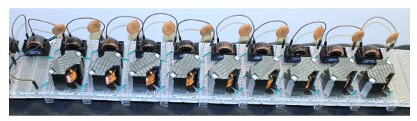
Figure 9: Electrical analogue of the cantilever beam with passive inductors, transformers and capacitors.
