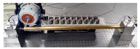
Figure 13: Experimental setup involving the beam coupled to its analogous electrical network.
