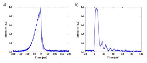
Fig. 3. a) evolution of the pulse amplification in the cavity. b) output pulse after reflection on the polarizer.
