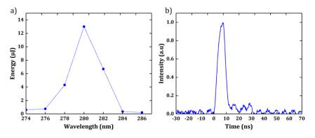
Fig. 7. a) Tunability of the UV pulses after THG: energy of the pulses versus the wavelength. b) output pulse in the UV.
