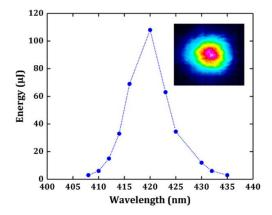
Fig. 6. Tunability of the blue pulses after SHG: energy of the pulses versus the wavelength. Insert: beam profile of the blue pulses.
