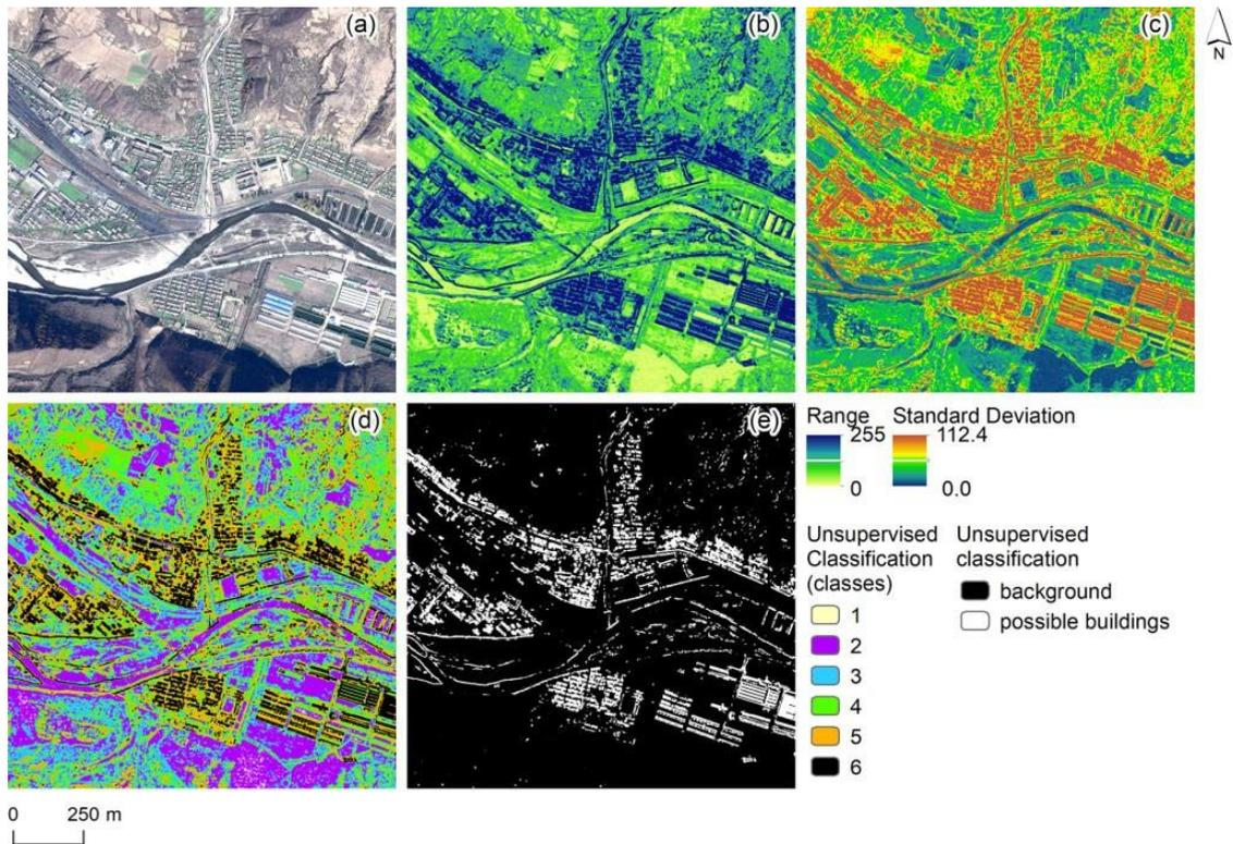
Figure 3. Example of satellite image, derived texture parameters and classification: (a) Pleiades 0.5 m satellite image; (b) local range of values (max–min); (c) local standard deviation of values within a 11 x 11 neighbourhood (Haralick, 1982); (d) iterative optimization clustering procedure implemented by the commercial software ArcGis® (Ball and Hall, 1965; Richards, 2013); (e) extracted buildings.
