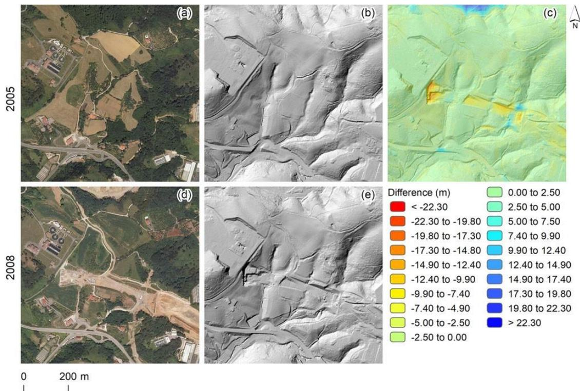
Figure 6. Example of change of detection from LiDAR Digital Terrain Model (DEM). Orthophotos for the year 2005 (a) and 2008 (d), LiDAR DEM in 2005 (b) and 2008 (e) and derived change of detection in m (c).
