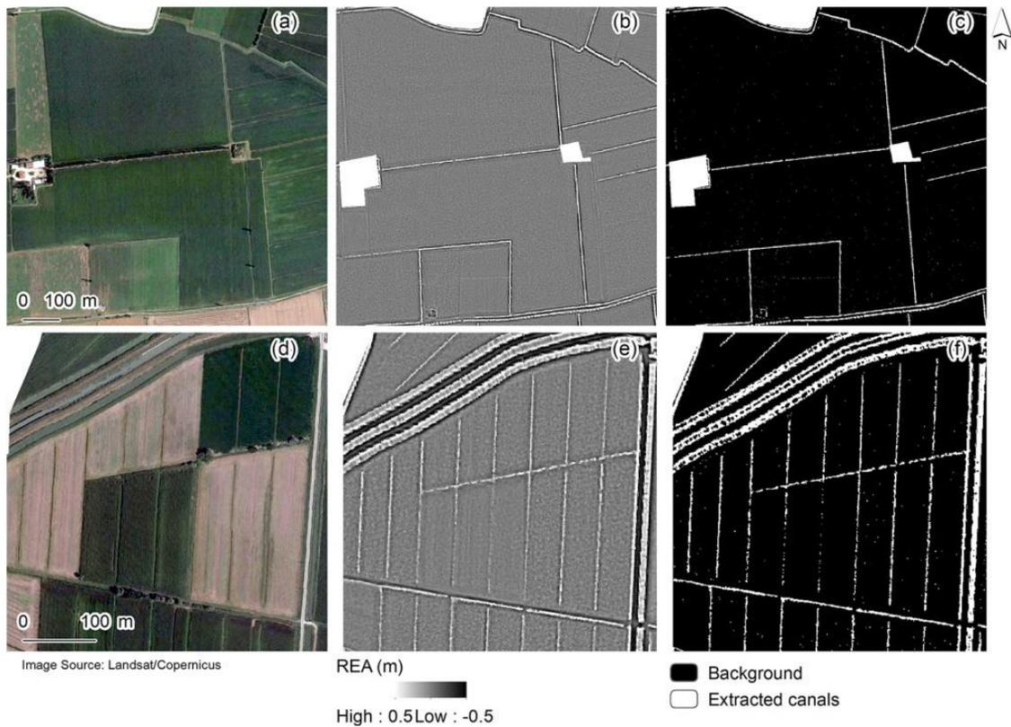
Figure 5. Agricultural practices in northeastern Italy ((a) tobacco; (d) corn). Detrended Digital Terrain Model (REMA, Cazorzi et al., 2013) (b), (e) and ditches derived automatically by applying a statistical threshold (standard deviation of Relative Elevation Attribute (REA)) (c), (f).
