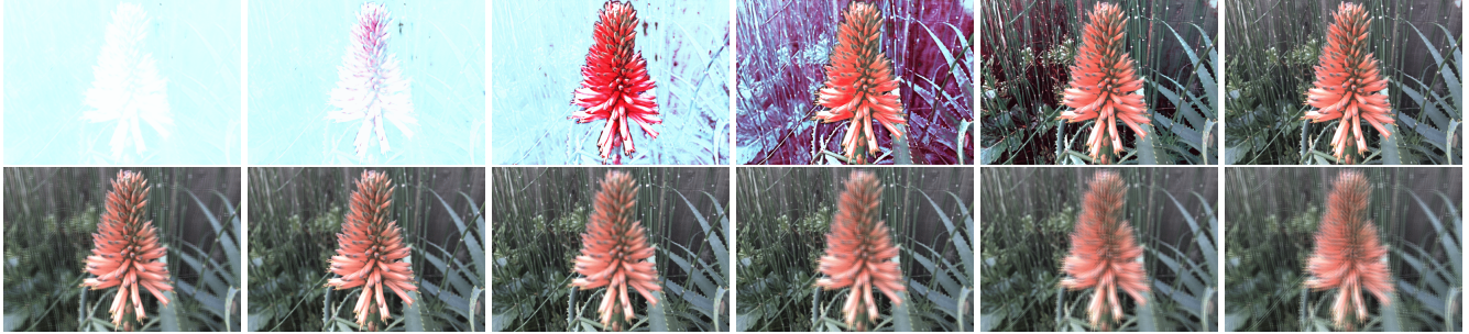
Fig. 2: Visualization of the LSTM state at different RNN iterations (to be read from left to right). On top we show the decoded memory state of the LSTM, on the bottom, we display the refocused 4 input views to see what depth plane is currently valid.
