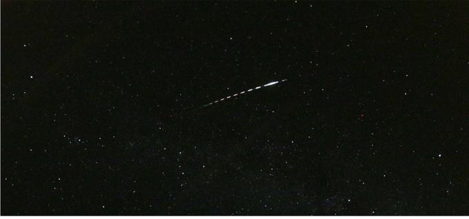
**Fig. 1.** Detailed view of the EN090916 SPE fireball recorded by the Digital Autonomous Fireball Observatory (DAFO) at the Czech station Kocelovice. The image of the fireball is interrupted by electronic shutter at a frequency of 16 Hz.
