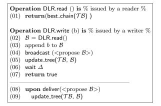
Fig. 1. DLR.read() and DLR.write() operations of the Safe Distributed Ledger Register.
