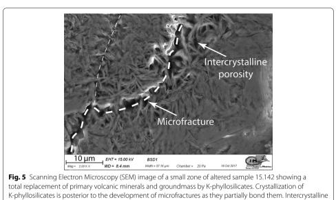
porosity is also encountered between K-phyllosilicate crystallites
