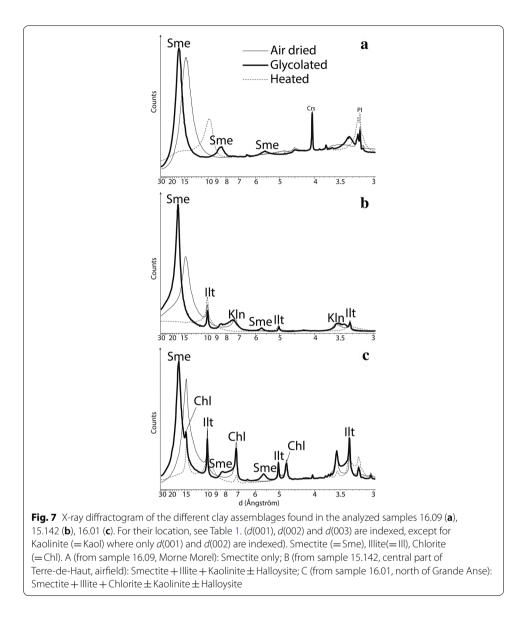
The third assemblage, which consists of smectite + chlorite + illite  $\pm$  kaolinite  $\pm$  halloysite (Fig. 7c), is only observed on the east side of the island, north of Grande Anse (Fig. 8), and is called the 'chlorite zone'. According to this study, this assemblage has the narrowest geographical distribution. The distribution of clay minerals allows us to distinguish the three different zones (Fig. 8).
