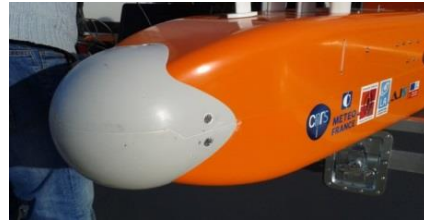
Figure 6: Picture of the five-hole probe on BOREAL
