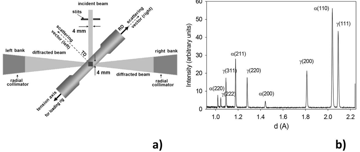
**Fig. 3.** The experimental setup (ENGIN-X instrument) used to measure relative lattice strains using neutron diffraction during *in situ* tensile tests (a). In figure (b) the TOF spectrum vs. inter-planar spacing  $d$  is shown and the diffraction peaks from  $\alpha$ -ferrite and  $\gamma$ -austenite are indicated (b).
