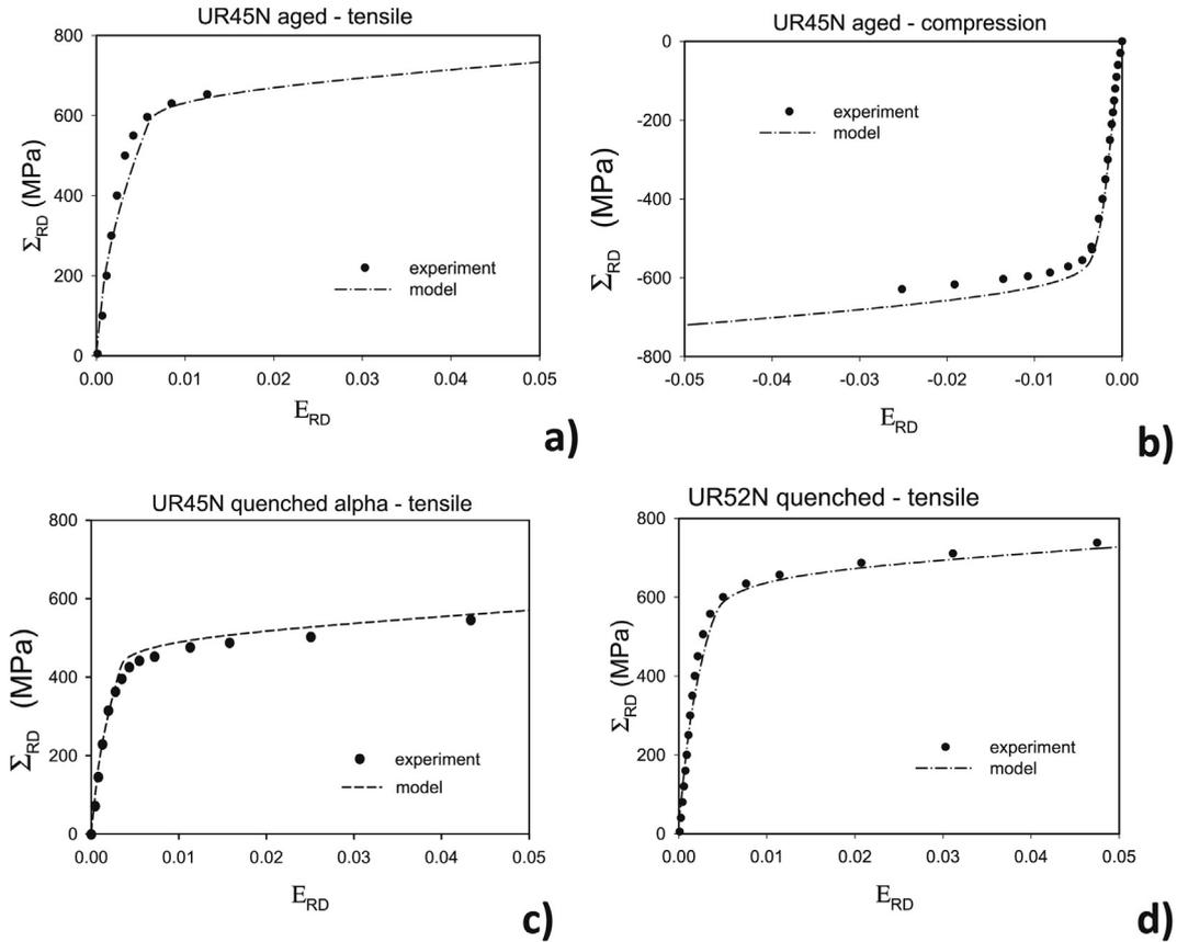
**Fig. 7.** Macro-mechanical stress  $\Sigma_{RD}$  vs.  $E_{RD}$  Plots for the aged UR45N steel subjected to tensile (a) and compressive tests (b); and for tensile tests performed on the quenched UR45N (c) and UR52N (d) samples. Experimental results (symbols) determined for small deformation range are compared with model simulations (lines).
