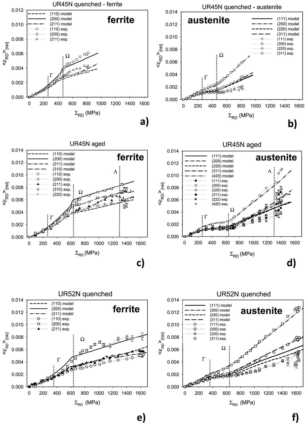
**Fig. 5.** Values of relative elastic lattice strains ( $\langle \epsilon_{RD} \rangle_{\{hkl\}}$ ) along the loading direction (RD) in function of the macrostress  $\Sigma_{RD}$  for quenched UR45N (a,b), aged UR45N (b,c) and quenched UR52N (e,f) samples. Experimental results (symbols) determined during tensile tests and results of model simulations (lines) are compared. The thresholds  $\Gamma$  and  $\Omega$  indicate the plastic yield of austenite and ferrite, respectively.
