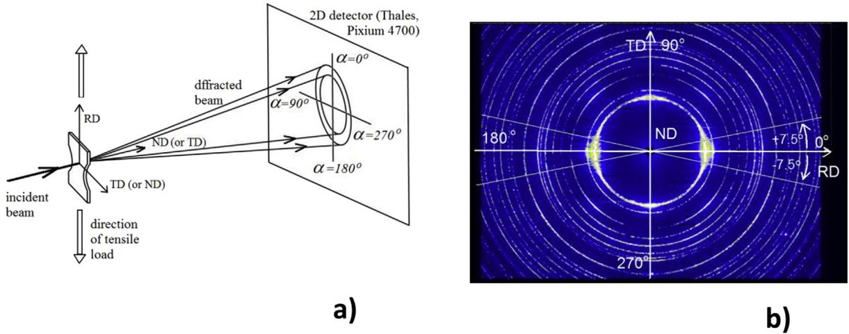
**Fig. 4.** The synchrotron diffraction experiment performed in the transmission mode at the beamline ID15B using a 2D detector (a) and an example of an image obtained on the CCD detector (b) are shown.
