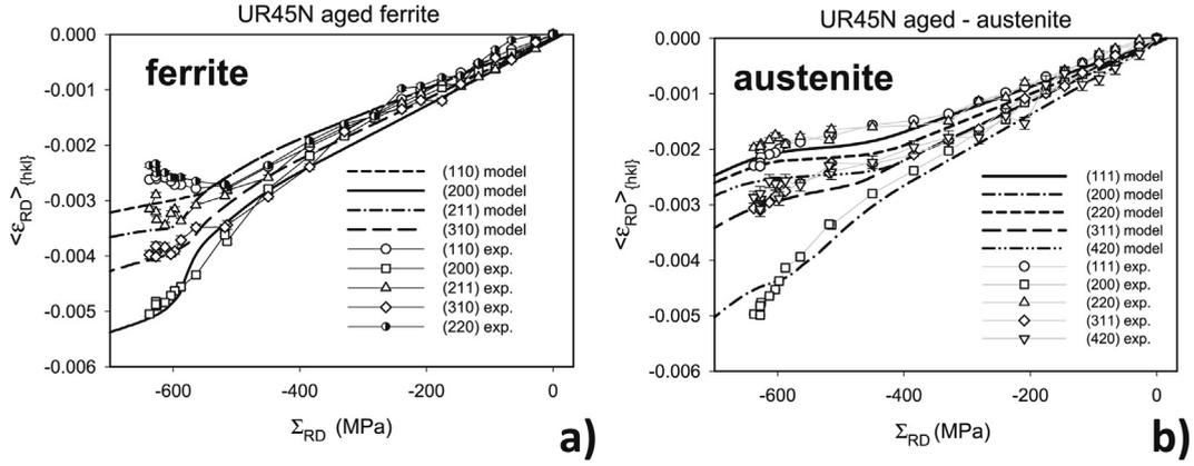
**Fig. 6.** Values of the measured relative lattice strains  $\langle \epsilon_{RD} \rangle_{\{hkl\}}$  vs.  $\Sigma_{RD}$  for the aged UR45N specimen (symbols) compared with the predictions (lines). The compressive test along RD was performed.
