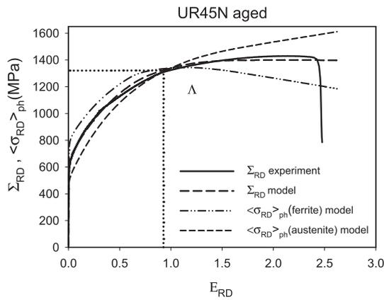
Fig. 11. The result of the tensile test conducted along RD compared with the model prediction. Additionally, the theoretical mean phase stresses  $\langle \sigma_{RD} \rangle_{ph}$  (along RD) in function of the total sample strain  $E_{RD}$  are presented. The  $\Lambda$  threshold indicates the approximate beginning of the damage process.
