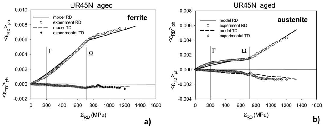
**Fig. 9.** Mean elastic phase strains vs. applied stress in the UR45N sample for a) ferrite and b) austenite. The experimental results (symbols) were measured along two directions (RD and TD) and compared with theoretically predicted lines (uncertainties are smaller than the symbols representing measured points). The thresholds  $\Gamma$  and  $\Omega$  indicate the yield points in austenite and ferrite, respectively.
