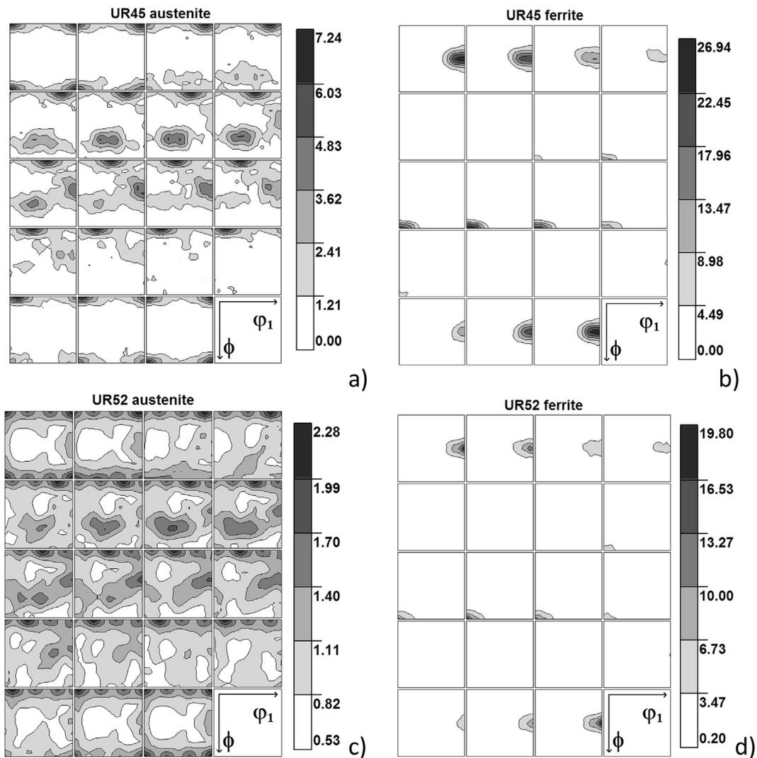
**Fig. 2.** Textures for austenitic (a,c) and ferritic (b,d) phases in the studied UR45N (a,b) and UR52N (c,d) steels. The ODFs are shown on the cross sections through Euler space, displaced with the increment of  $5^\circ$  along the  $\varphi_2$  axis (Kallend et al., 1990). The sample orientation is defined through:  $x_1 \parallel$  TD,  $x_2 \parallel$  ND and  $x_3 \parallel$  RD.
