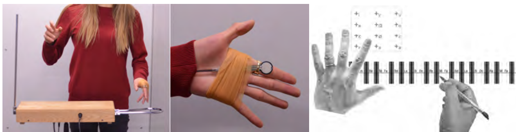
Fig. 1. T-Voks (Theremin + button, right) & C-Voks (stylus/tablet + button/surface, left)
