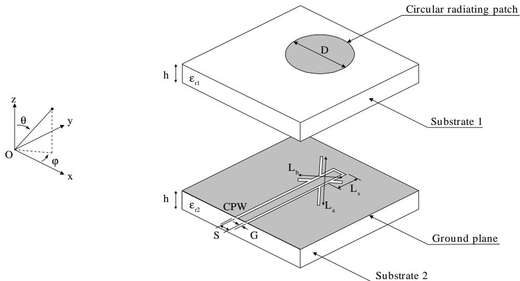
Fig. 1: Geometry of the circularly polarized microstrip antenna using asymmetrical cross coplanar slot ( $D = 9.2$ mm,  $\epsilon_{r1} = 2.2$ ,  $\epsilon_{r2} = 4.5$ ,  $h = 1.6$ mm,  $S = 1.2$ mm,  $G = 0.2$ mm,  $L_s = 2.1$ mm,  $L_a = 8.6$ mm,  $L_b = 4.3$ mm).
