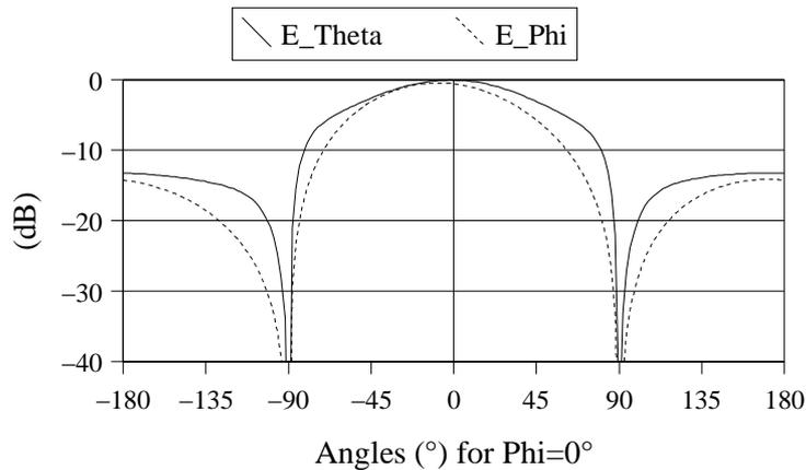
Fig. 4: Simulated radiation patterns at 11.74GHz.
