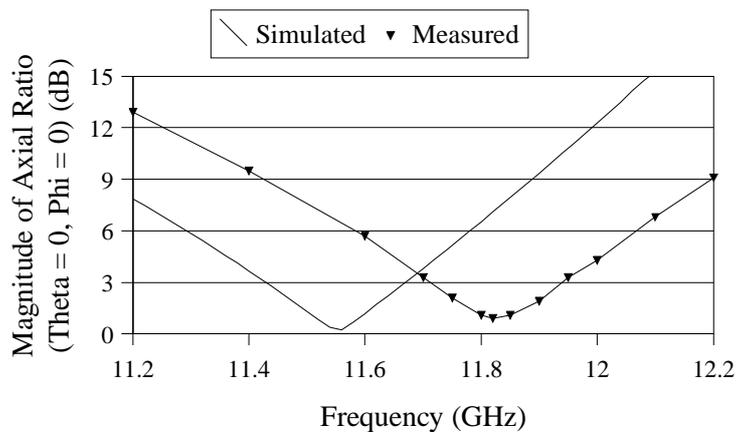
Fig. 5: Simulated and measured axial ratio versus frequency.
