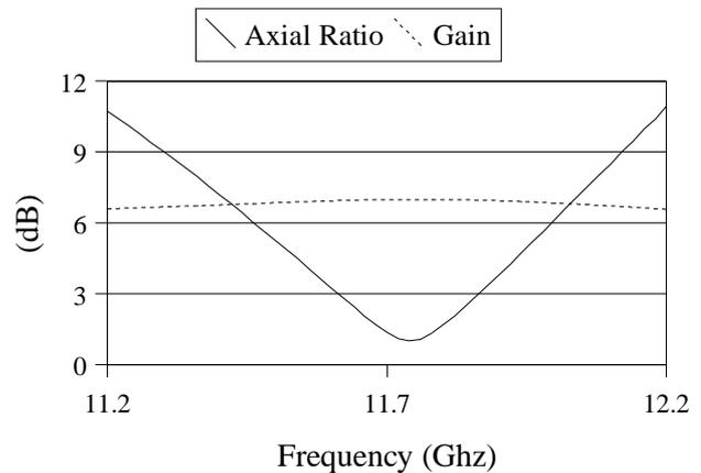
Fig. 3: Simulated axial ratio and gain versus frequency.
