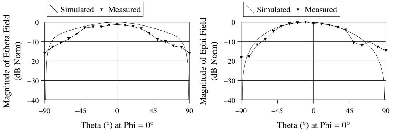
Fig. 6: Simulated and measured radiation patterns.
