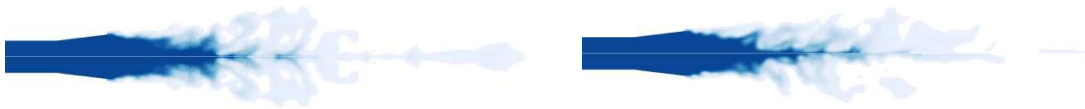
Figure 6: iso-values of liquid volume fraction with atomization (upper side of the axis) and without atomization
