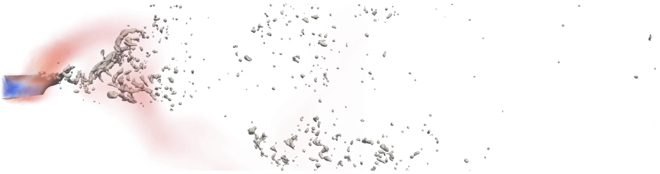
Figure 10: Instantaneous liquid core comparison. CEDRE: volume rendering of the liquid volume fraction, \alpha_{H_2O} high low, grey isosurface \alpha_{H_2O} = 0.99 . ARCHER: Grey isovolume of liquid volume fraction \alpha_{H_2O} = 1
