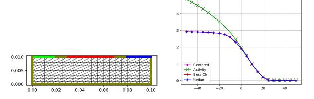
FIGURE 9. Discretization grid of refinement level  $n_{ref} = 1$  (left) and corresponding I-V curves for different discretization schemes (right).
