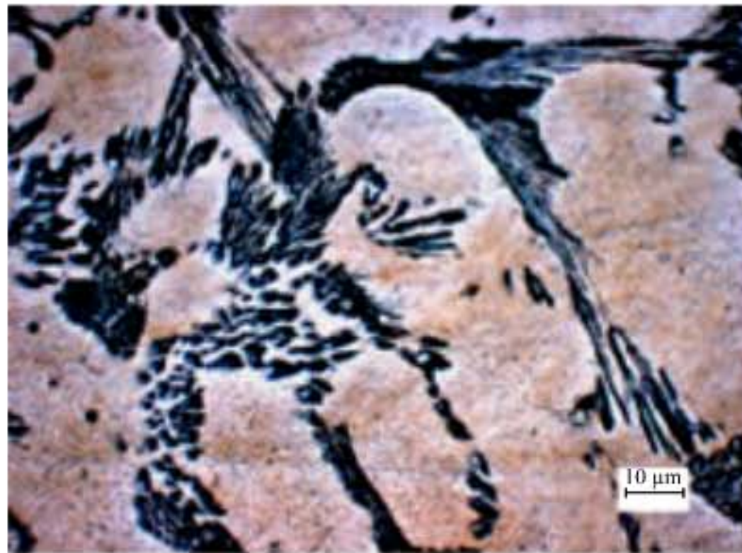
Fig. 6: Optical micrograph showing microstructure of infiltrant after sintering (attacked with Nital)
