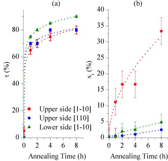
Figure 4. Evolution of the transformation level  $\tau$  (a) and the the volume fraction  $x_t$  (b) as function of annealing time at 2000°C. Squares: upper side, high SF density [1-10]; circles: upper side, low SF density [110]; triangles: lower side. The dotted line is a fit with a power-law.
