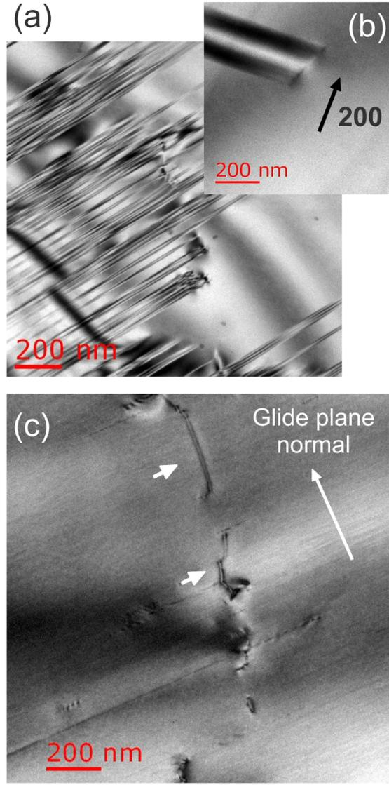
Figure 6. (a) Bright-field TEM image showing a region with a high density of large stacking faults lying in  $\{111\}$  in annealed 3C-SiC. (b) Detail of one stacking fault and the associated bounding partial dislocation. (c) Bright-field image of another area showing dislocation segments lying out of the  $\{111\}$  primary glide plane in a plane-view sample.
