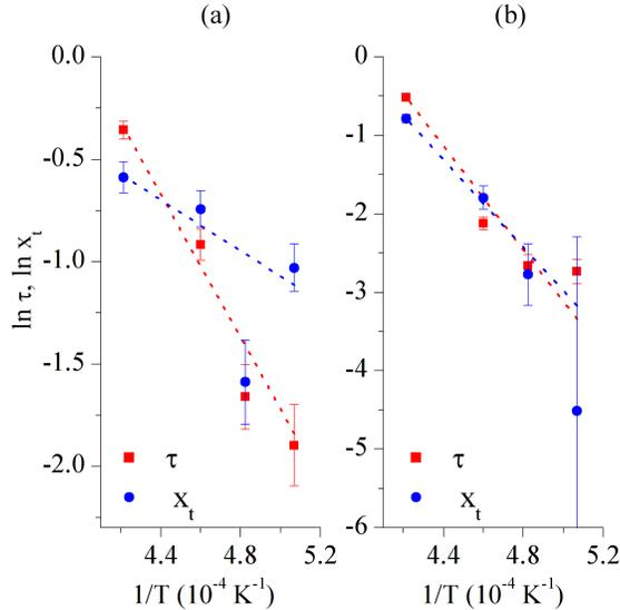
Figure 5. Arrhenius plot of the transformation level  $\tau$  (squares) and volume fraction  $x_t$  (circles) obtained from the upper side (a) and the lower side (b).
