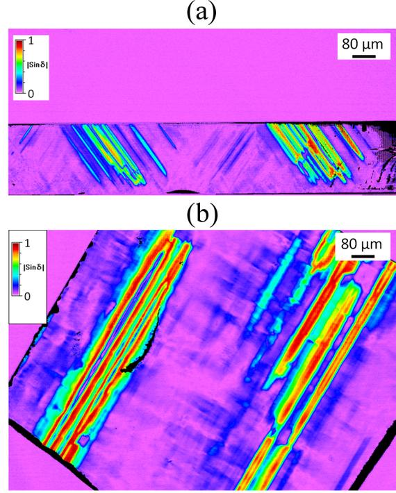
Figure 2. Optical birefringence micrograph of a partially transformed 3C-SiC single crystal. (a) cross-sectional view, (b) plane view.  $\delta$  is the magnitude of birefringence ( $\delta = 0$  corresponds to cubic regions, and  $\delta > 0$  corresponds to regions with non-zero hexagonality, i.e. partially transformed regions)
