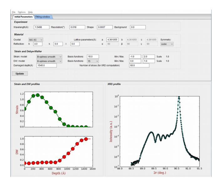
Fig. 3. Screenshot of RaDMaX running in Windows 10. The simulation corresponds to irradiated silicon carbide.
