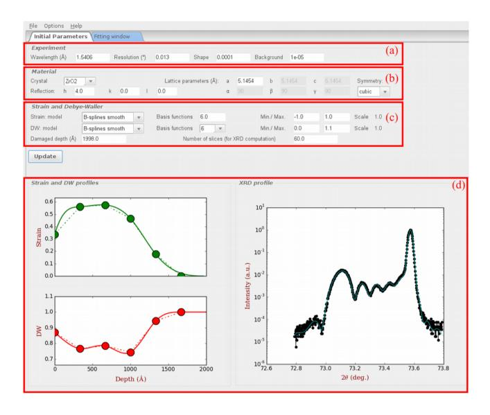
Fig. 1. Screenshot of RaDMaX running in Kubuntu 15.04. The simulation corresponds to irradiated yttria - stabilized zirconia.
