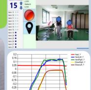
Kinect data recorded are converted into biomechanical observables on kinematic graphs and 3D reconstruction allowing the item scoring using different data (angles, distances...)
