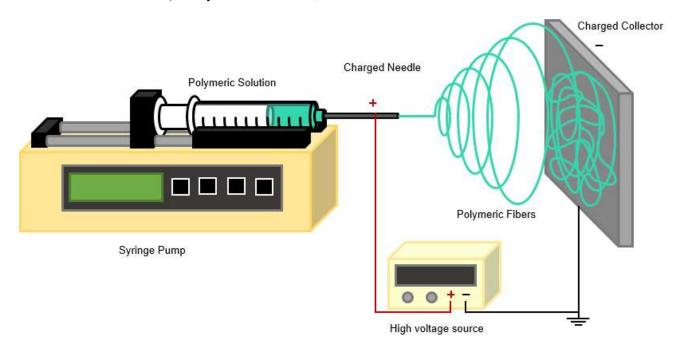
Figure 1. Basic diagram of the electrospinning device.
