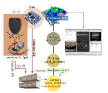
Fig. 17: The 2D to 3D LiDAR transformation concept
