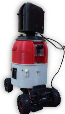
Fig. 11: Realised Test Robot with LiDAR3D mounted.
