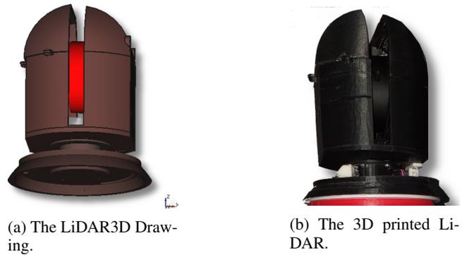
Fig. 10: The LiDAR 3D model.
