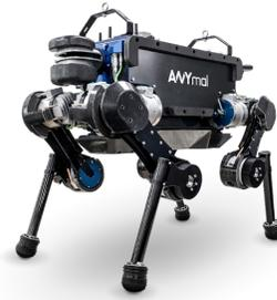
Fig. 14: Robot ANYmal, ETH/Robotics [12], [31], [7].
