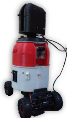
Fig. 11: Realised Test Robot with LiDAR3D mounted.
