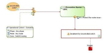
In this case, the preventive barrier is constituted of elements of the system. Thanks to tool integration, safety engineers can directly use elements of the SysML model during their analyses.
