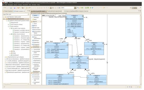
Safety engineers can start risk assessment with the preliminary risk analysis. Accidental scenarios are graphically defined as in figure: a safety hazard "Uncontrolled switch" is defined in a given context, the preventive barrier CBTC and its function "F3: Protect the route issues" prevent from the accident "Derailment by uncontrolled switch" and its consequence "Injuries".
