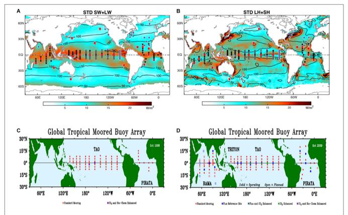
**FIGURE 3** Standard deviation of the means based on 14 products for **(A)** SW + LW and **(B)** LH + SH for the 10-year period of 2001–2010. Black contours denote the ensemble mean patterns. The location of the global moored surface buoys is superimposed, with red dots indicating flux reference moorings (adapted from Yu, 2019). Detailed instrumentation of the Tropical moored buoy array in panel **(C)** 1990 and **(D)** 2009 (from McPhaden et al., 2010).
