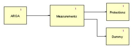
Figure 8. Root node of the SCADE model of the Sepam application.
