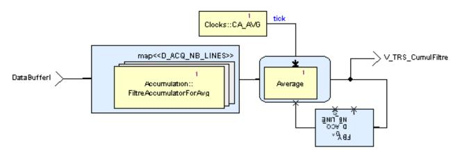
Figure 10.  ${\bf AgentAverage}$  node of the SCADE model of the Sepam application.
