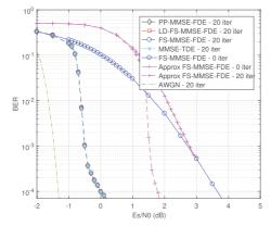
Fig. 2. BER over the aeronautical channel by satellite.
