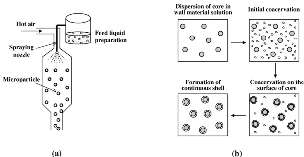
**Fig. 2.** Schematic representation of microencapsulation process by spray-drying (a) and coacervation (b) techniques. (Redrawn from Jyothi et al., 2010).
