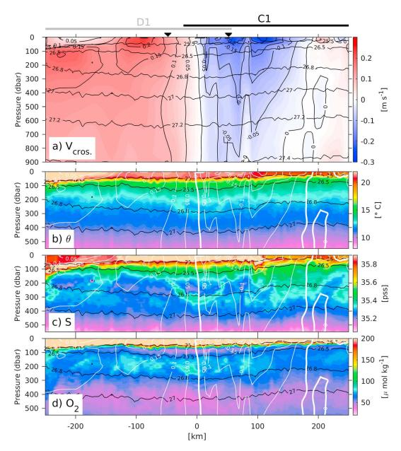
**Figure 3.** (a) Composite geostrophic meridional velocities (in m/s<sup>-</sup>) computed between 0 and 900 dbar and 23–18°W; (b) composite potential temperature (in °C); (c) composite salinity (in psu); (d) composite dissolved oxygen (in  $\mu$ mol/kg) between 0 and 550 dbar and 23°W–18°W reconstructed from D1 and C1. Parameter  $\sigma_{\theta}$  = 25.5; 26.5; 26.8; 27 kg/m<sup>3</sup> contours are superimposed (solid thin black).
