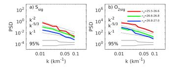
**Figure 9.** Density power spectra of isopycnal salinity (a) and odissolved oxygen (b) between 18°W and 23°W (C1, C2, D1 sections) within the  $\sigma_{\theta} = 25.5$ –26.6 (red), 26.6–26.8 (green), and 26.8–27 (blue) kg/m³ isopycnal layers. The  $k^{-1}$ ,  $k^{-5/3}$ , and  $k^{-2}$  slopes are superimposed (dashed lines). The 95% confidence interval is indicated by gray solid lines.
