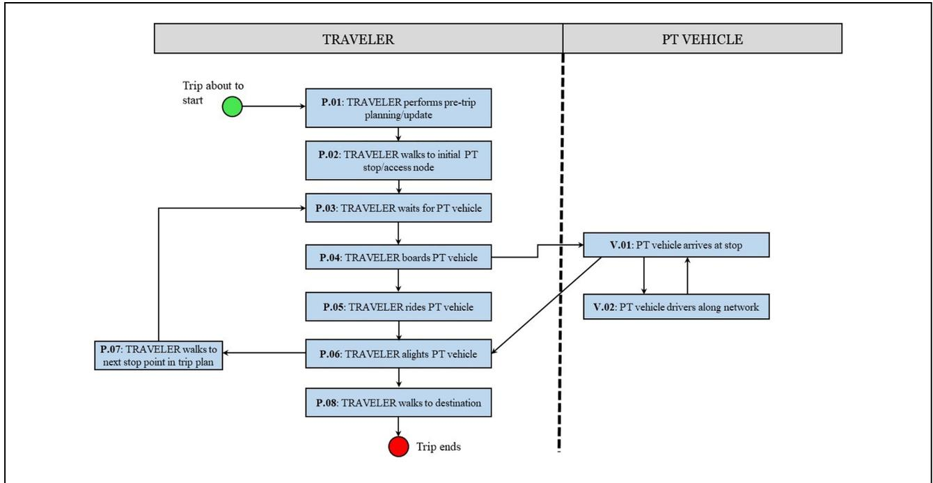
**Figure 6.** Traveler movement: stages of a transit trip.
