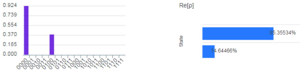
Figure 87 On the left, the wavefunction’s complex modulus. On the right, the real part of the state.
